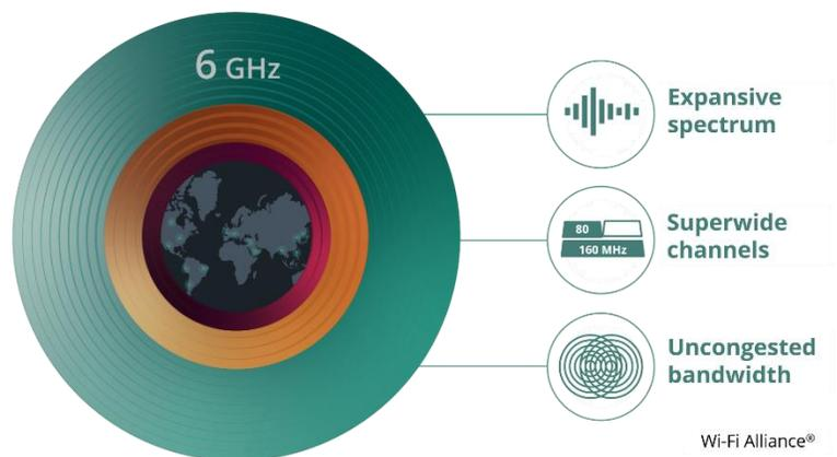
6 GHz brings additional spectrum capacity through contiguous spectrum blocks, which accommodate 14 additional 80 MHz channels or seven additional 160 MHz wide channels. Wi-Fi 6E utilizes the less congested 6 GHz band to enable high-bandwidth applications that require faster data throughput, as well as lower latency connectivity that is specifically well suited for next generation uses, such as unified communications, cloud computing, augmented and virtual reality, and telepresence.
