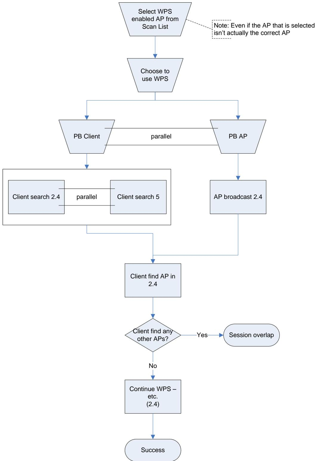
Figure 7 – Scenario 4: PBC from Scan List on Client, Client = 2.4 GHz / 5 GHz, AP = 2.4 GHz
