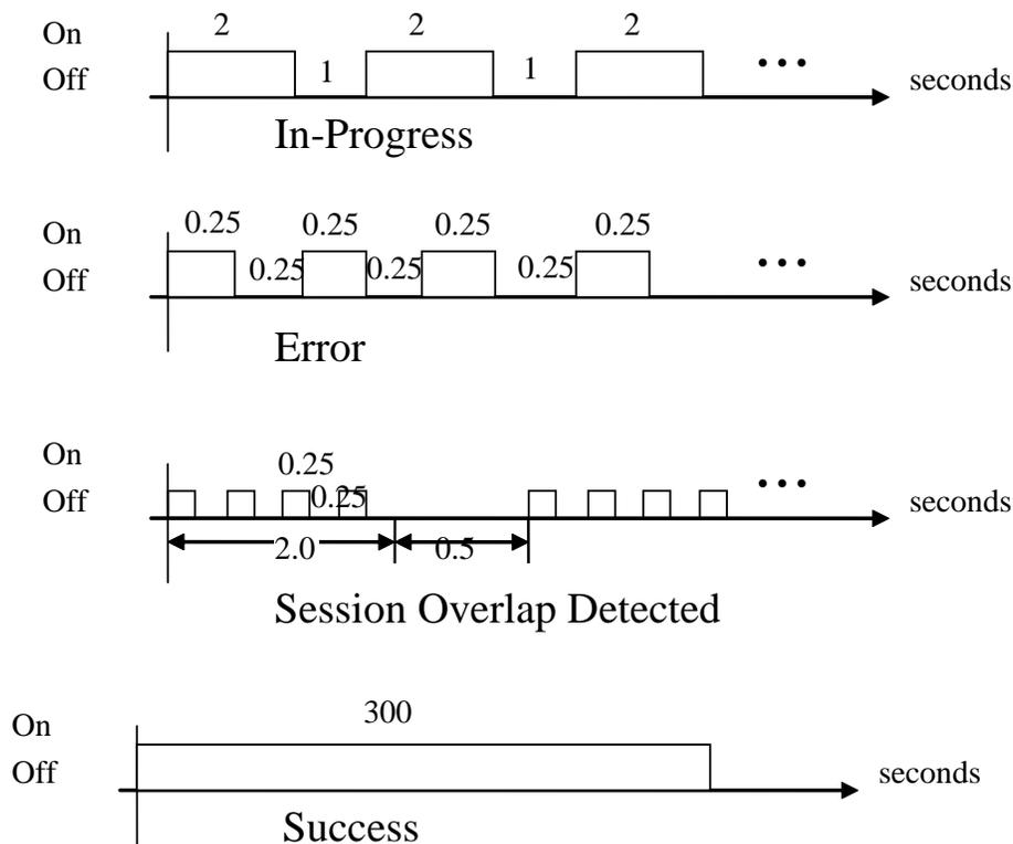
Figure 1 – WSC Visual Indicator LED Flashing Frequencies
